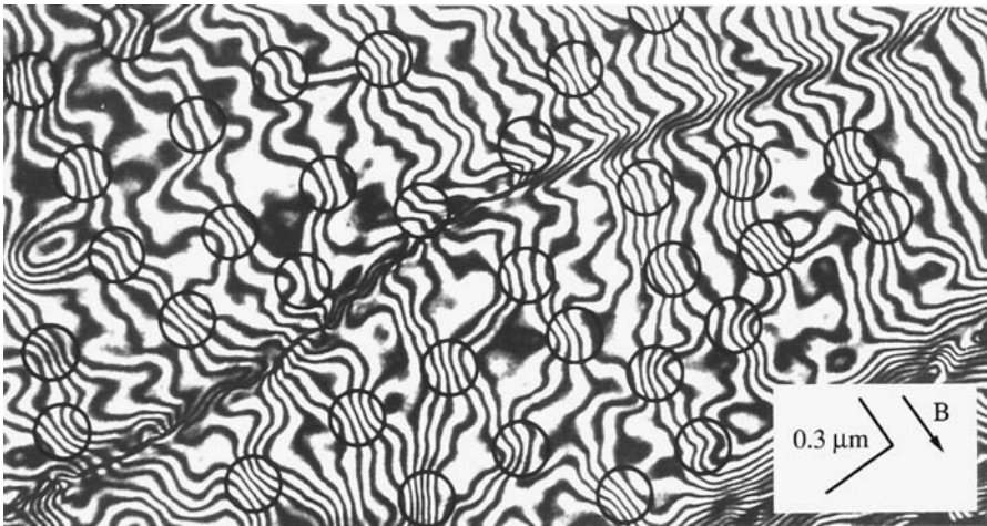
Fig. 6.43. Reconstructed hologram of vortices (magnetic flux lines with \Phi_m = h/2e ) in a superconducting 70 nm niobium foil inclined by 45^\circ in a 300 kV transmission electron microscope [6.286].
