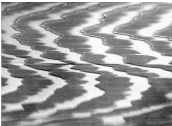
Fig. 9.42. Reflection electron microscope (REM) image of the (111) face of an Si crystal obtained with the (444) diffracted beam and showing the nucleation and growth of 7\times 7 structures (dark regions) at surface steps when the specimen is cooled from the transition temperature at 830°C, where it shows the 1\times 1 structure (bright regions) (courtesy of H. Yagi).
