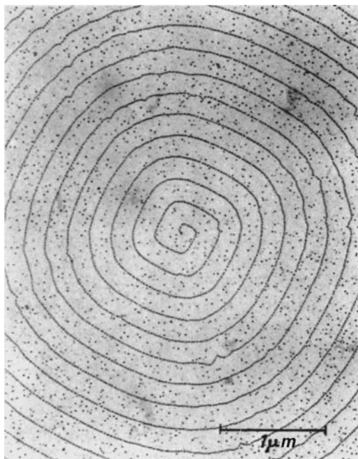
Fig. 9.37. Surface replica of a deformed copper single crystal (8% stretched). The mean step height is 1.8 nm. The carbon film is reinforced with a collodium backing and shadowed with a palladium film (courtesy of S. Mader).
